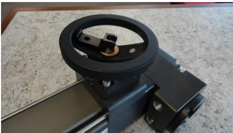
Handwheel in Engaged Position (Step 3)
