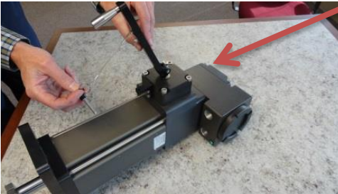
Remove Pin and Flip Hand Crank (Steps 2 & 3)
