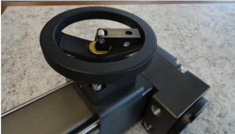
Handwheel in Disengaged Position
