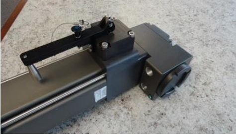
Hand Crank in Disengaged Position
