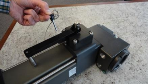
Hand Crank in Disengaged Position
